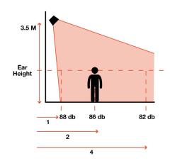
Carefully planning your audio coverage and loudspeaker spacing is key to any successful loudspeaker design.
