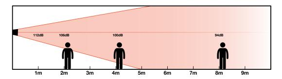
In the above example the loudspeaker can deliver II2dB at Im and thus 94dB at 8m, which is above the 84dB desired level, so the loudspeaker can do the job.
