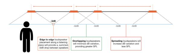
In applications with very high ceilings a single loudspeaker may cover too wide an area. Control Contractor offers the Control 47HC, a specially designed ceiling loudspeaker with a much narrower wave guide, so the energy covers a smaller area. Alternatively there is also a series of Control Contractor Pendant loudspeakers so you have the option of hanging them at a height that is closer to the listeners.
